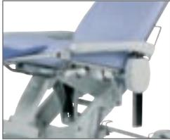
A handle under the armrests lowers them to the same level as the seat for easier transfers. The height of the armrests can be adjusted on a 6-position rack mechanism with 240 mm of travel for perfect two-handed transfer.
